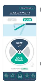
To lower the gate, hold the **DOWN** button for 3 seconds on the remote. (Full gate drop can take 8-15 minutes - time varies depending on water conditions)
